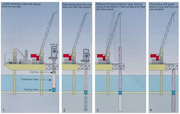
Figure 2.1-1. Monopile foundation installation sequence.
