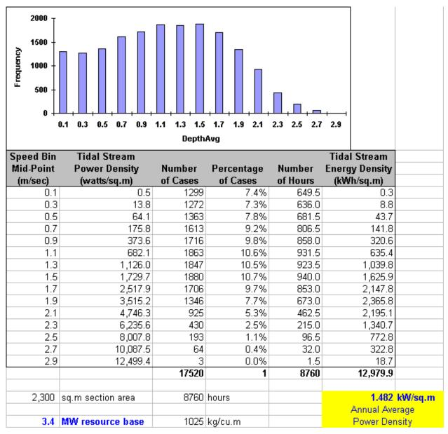
Figure 3.10-2. Tidal in-stream power density histogram for Piscataqua River.
