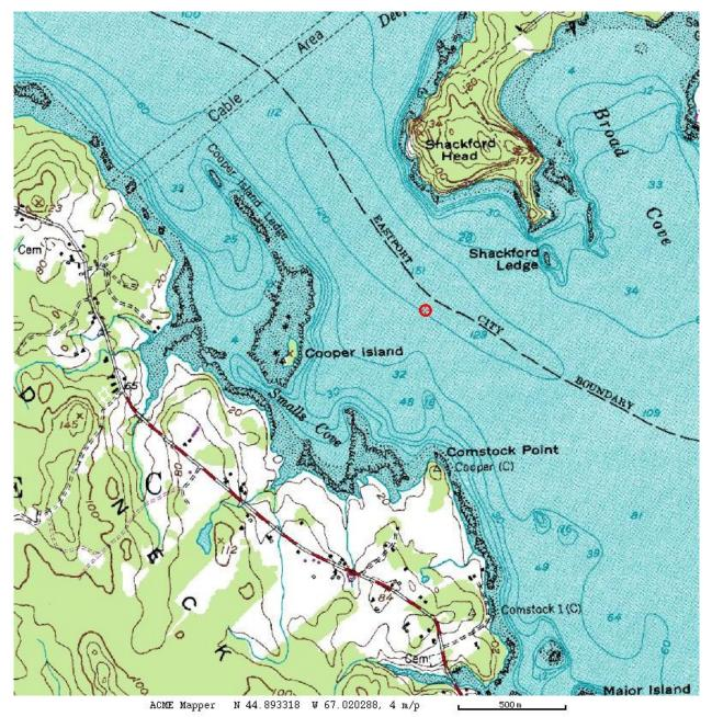
*Figure 3.3-4. Bathymetric chart of Outer Cobscook Bay off Shackford Head and Goose Island. Red circle indicates location of GoMOOS monitoring buoy, Station J (Source: Reference 7).*
