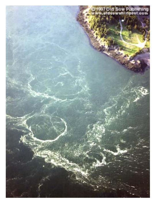
Figure 3.2-2. Aerial photo of Old Sow tidal whirlpool, with Deer Island Point at upper right. The 90° collision of the flood current out of Indian River (coming from right side of photo) and the flood current in Western Passage (heading toward left side of photo) is clearly visible.
