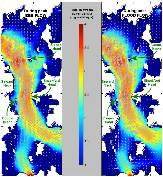
Figure 3.3-2. Tidal in-stream power density, mapped as the base-10 logarithm of watts per square meter of flow cross-sectional area, during peak ebb and flood in Outer Cobscook Bay, under average tidal conditions. Note that there are two centers of maximum power density in this channel: between Shackford Head and Cooper Island Ledge, and due south of Goose Island, where the flow is constricted before it bends around Seward Neck (Reference 17).
