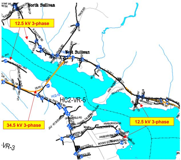
Figure 3.4-4. BHE utility grid in West Sullivan (Source: Bangor Hydro-Electric Company).
