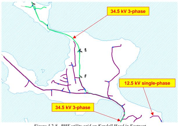
Figure 3.2-8. BHE utility grid on Kendall Head in Eastport (Source: Bangor Hydro-Electric Company).
