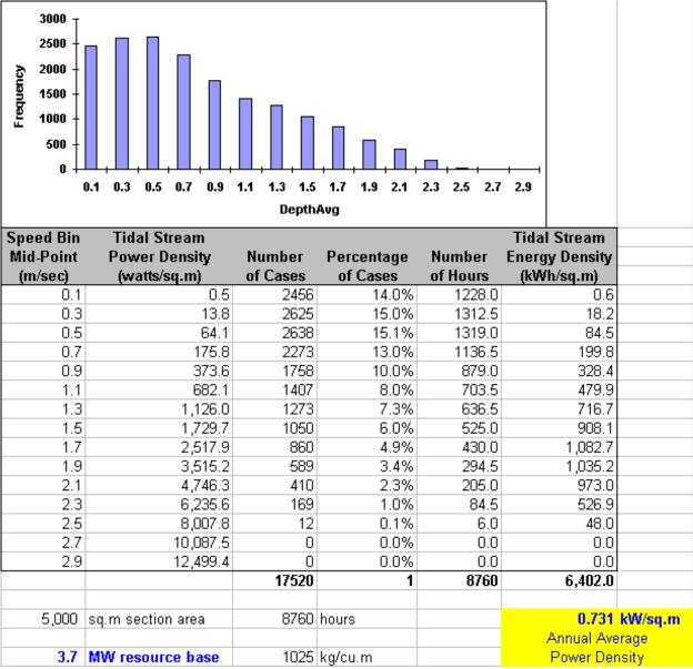
Figure 3.6-2. Tidal in-stream power density histogram for Penobscot River.
