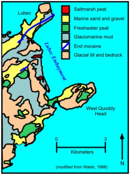
*Figure 3.1-6. Geologic map of shoreline bordering the Lubec Embayment between Lubec Neck and West Quoddy Head (Source: Reference 9).*
