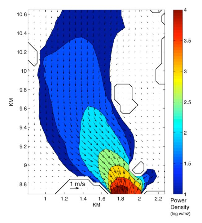
Figure 3.1-3. Tidal in-stream power density, mapped as the base-10 logarithm of watts per square meter of flow cross-sectional area, during peak ebb flow in Lubec Narrows, under average tidal conditions. Note that the peak ebb power density is on the order of 10 kW/m<sup>2</sup> on the American side, compared to 3 kW/m<sup>2</sup> on the Canadian side (Reference 1).
