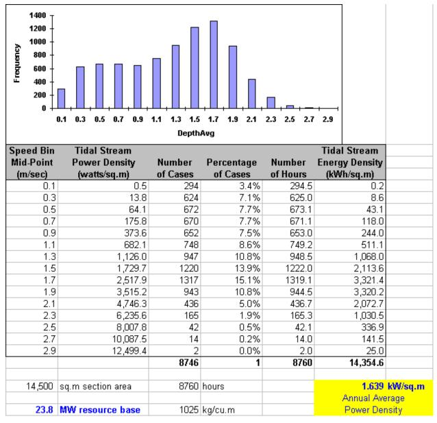
Figure 3.3-3. Tidal in-stream power density histogram for Outer Cobscook Bay.
