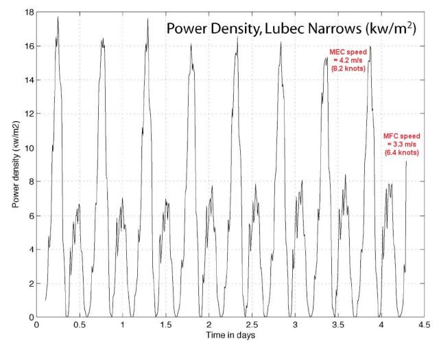
*Figure 3.1-2. Tidal in-stream power density in Lubec Narrows under average tidal conditions. Maximum Ebb Current (MEC) speed averages 8.2 knots, and Maximum Flood Current (MFC) speed averages 6.4 knots, but respective power densities differ by a factor of two (Reference 1).*
