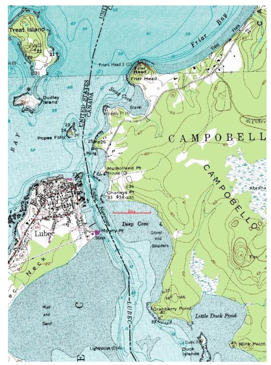
Figure 3.1-4. Bathymetric chart of Lubec Narrows and Lubec Channel as far south as Duck Islands. Note 200 m long deep area between Mulholland Pt. and Charleys Pt., and 800 m long deep area from beneath the Roosevelt Memorial Bridge, extending 300 m south of Mowry Pt. (Reference 7).
