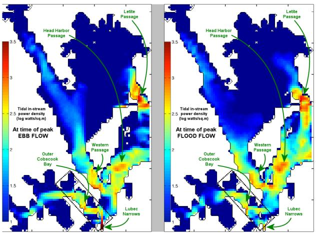
Figure 3.2-3. Tidal in-stream power density, mapped as the base-10 logarithm of watts per square meter of flow cross-sectional area, during peak ebb and flood in Passamaquoddy and Cobscook, under average tidal conditions. Note that where Western Passage widen, north of its narrow entrance, the tidal in-stream power density drops by one-half to one order of magnitude (Source: Reference 18).
